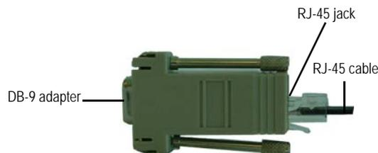
2. Plug the male end of the RJ-45 CAT5 serial cable into the Console port on the SSG 5. (Be sure that the other end of the CAT5 cable is inserted properly and secured in the DB-9 adapter.)
