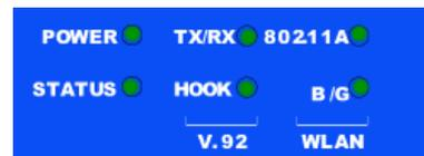
When the system powers up, the POWER LED changes from off to blinking green, and the STATUS LED changes in the following sequence: red, green, blinking green. Startup takes approximately two minutes to complete. If you want to turn the system off and on again, we recommend you wait a few seconds between shutting it down and powering it back up. Table 2 provides the type, name, color, status, and description of each system status LED.
