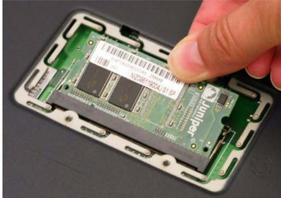
8. Insert the 256 MB DIMM DRAM into the slot. Exerting even pressure with both thumbs upon the upper edge of the module, press the module downward until the locking tabs click into position.
