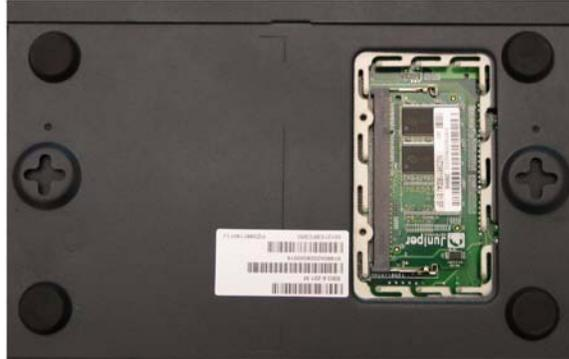
6. Release the 128 MB DIMM DRAM by pressing your thumbs outward on the locking tabs on each side of the module so that the tabs move away from the module.
